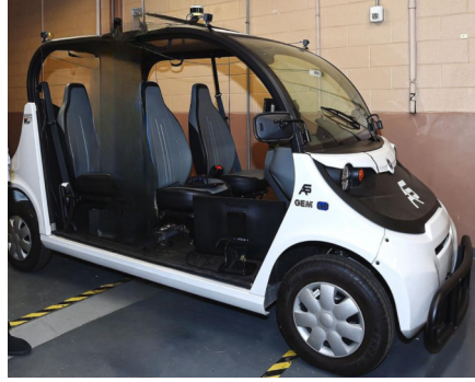
Fig. 6. The testbed includes a Polaris GEM e4 electric vehicle equipped with Sekonix cameras for face monitoring. The on-vehicle processing unit is the NVIDIA Jetson AGX Xavier.
