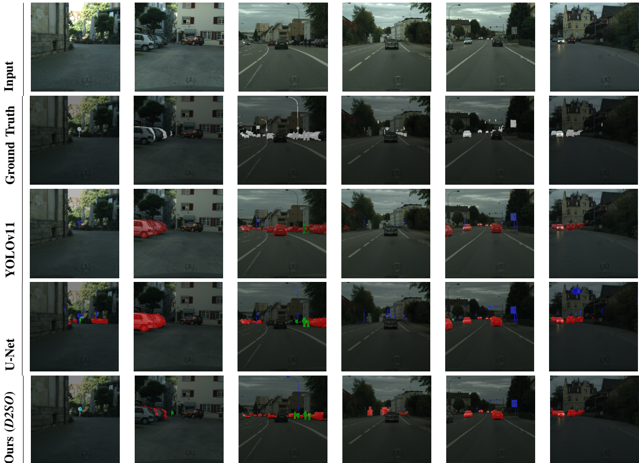
Fig. 3: This collage displays six samples, each consisting of three panels: input images, ground truth images, and predicted images. In these samples, D2SO specifically targets the detection of distant objects, defined as those smaller than 24 \times 24 pixels in size. The predicted outputs are color-coded to enhance clarity: vehicles are marked with red, static structures with green, and humans with blue. This visual representation emphasizes the model’s capability to accurately identify and differentiate between various object classes at a distance.
