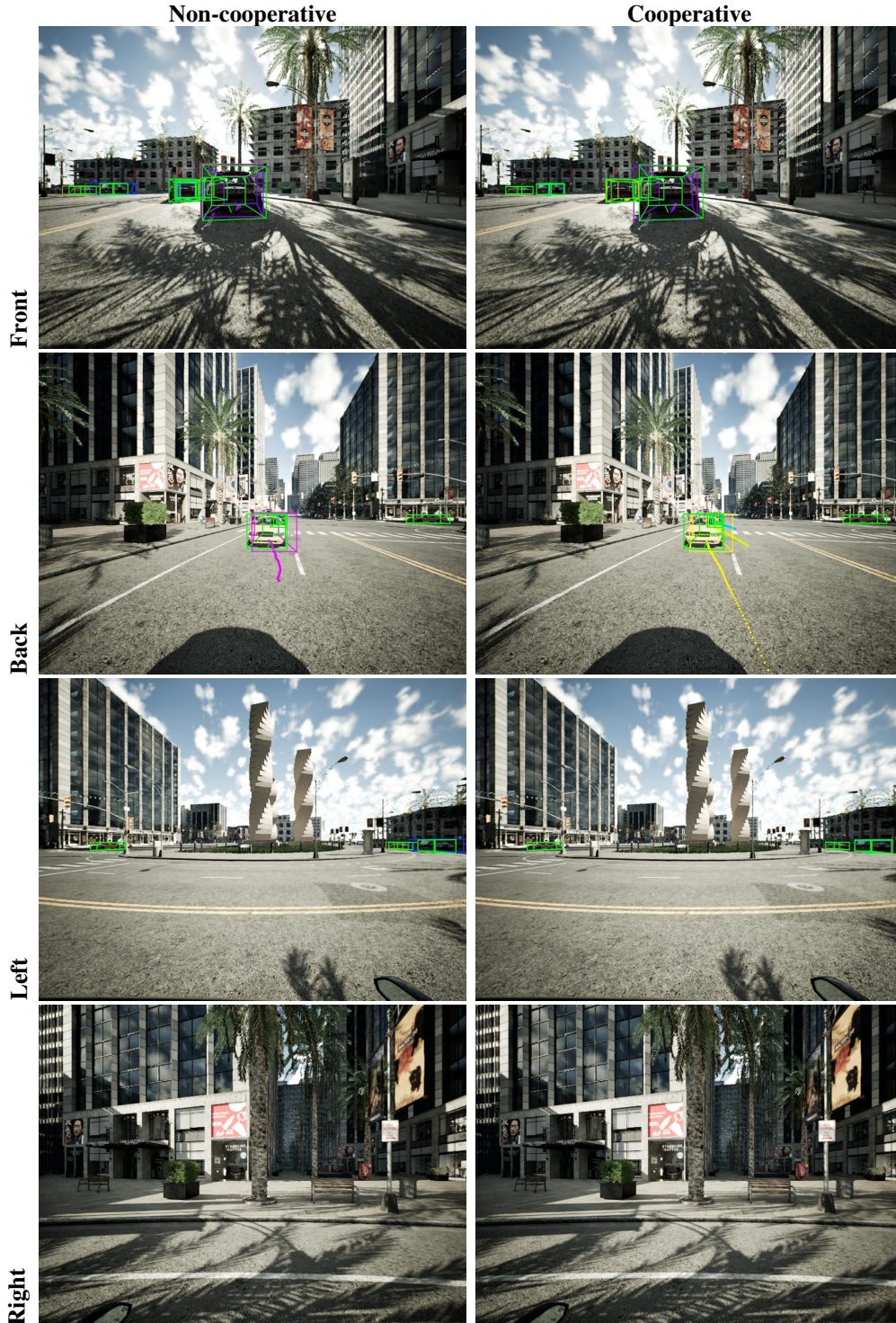
Figure 12: Rows list the camera view (front, back, left, right), columns compare the performance of single vehicle against the cooperative solution, showing the differences in object detection and motion forecasting results from different viewpoints.
